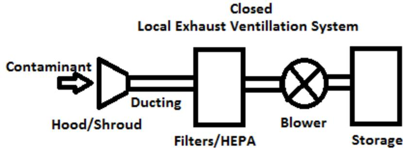
LEV is an engineering system designed to reduce employee exposure to airborne contaminants (dust, mist, fume, vapor, gas) in the workplace by capturing the emission at source and transporting it to a safe emission point or to a filter/scrubber.<sup>1</sup>
